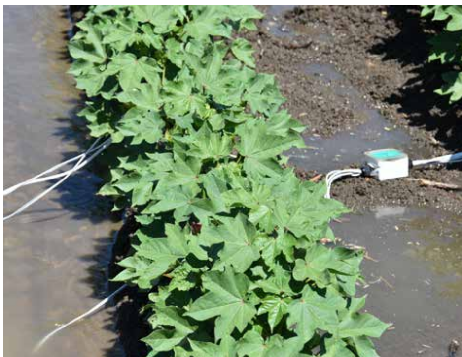
Irrigation advance sensors being used in the Gwydir Valley, Moree.
