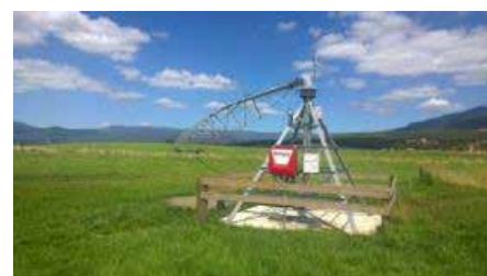
Variable rate irrigation system used with VARIwise prescription maps.
