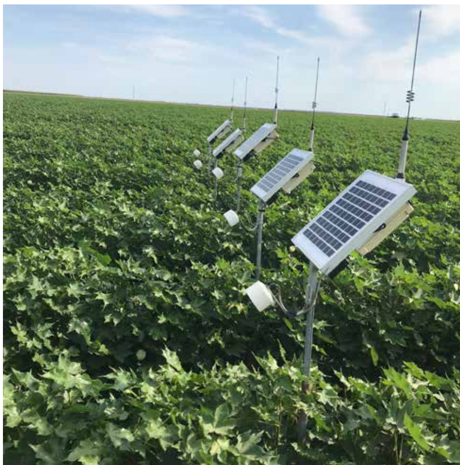
Solar powered canopy temperature sensors in a cotton crop.
