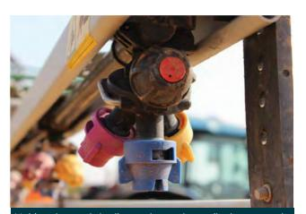
Multi-outlet nozzle bodies can be used to easily change nozzle types across a boom, or operate multiple nozzles in differing directions to increase coverage. Ensure that spray equipment has been recently calibrated and poorly performing nozzles have been replaced.
