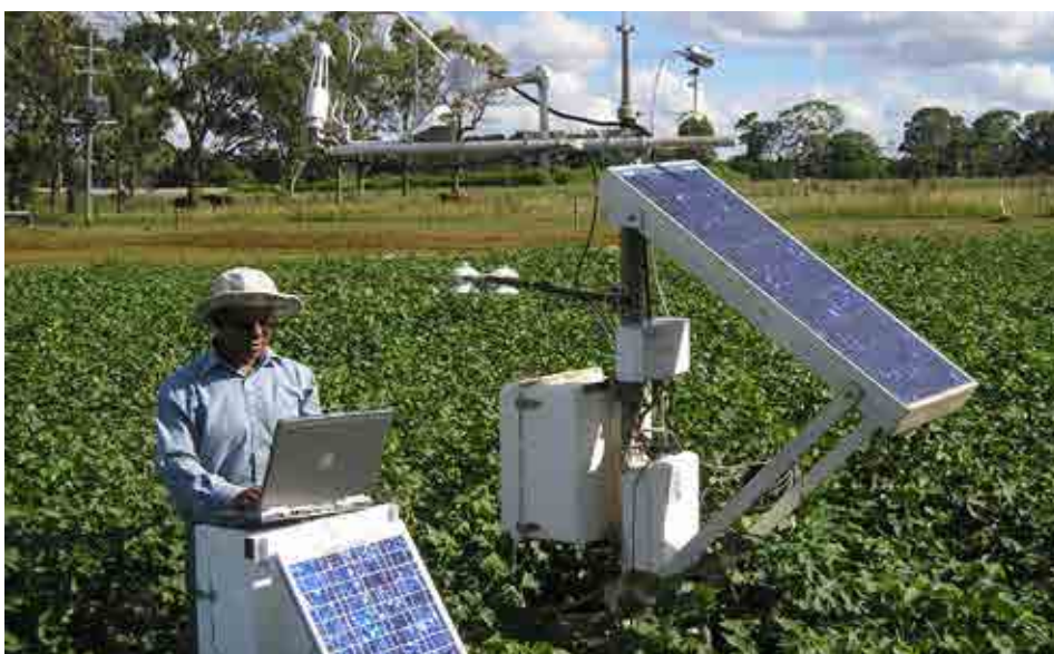
FIGURE 1. Installed ECV and sap flow system at the centre of the field for continuous measurements
