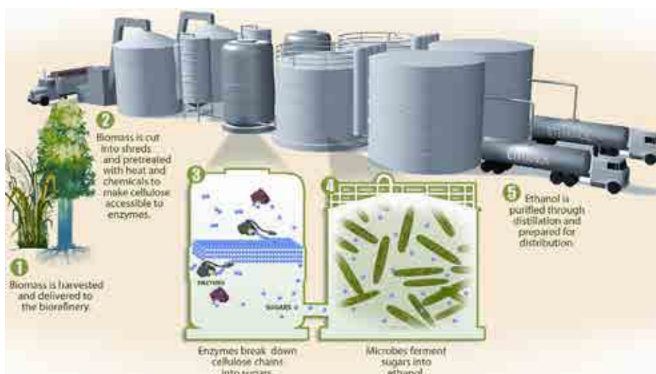
FIGURE 1. Lignocellulose to ethanol conversion steps. (1) Biomass harvesting and delivery. (2) Thermal and/or chemical pretreatment separates cellulose from lignin seal and exposes it to enzymatic digestion. (3) Enzyme mix is added to digest cellulose into simple sugars. (4) Microbes produce ethanol by fermenting recovered sugars. (5) Ethanol is distilled and concentrated. Graphics by U.S. DEG Programs ( http://genomics.energy.gov ).
