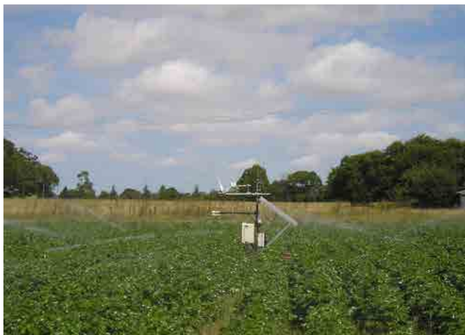
FIGURE 2. Evapotranspiration being measured during irrigation with the ECV system
